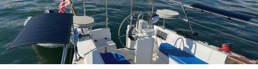
Paper-thin profile measures just 3/8" (9mm), with curvature allowing for optimal solar efficiency and snag-free operation.
